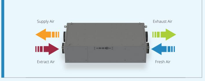
Heat recovery units are used to reduce the energy required to heat or cool the buildings. This is done by recovering the residual heat of the exhaust air and transferring it to the supply air by the means of heat exchangers. BSK BRHU Plus units use high thermal efficiency heat exchangers to transfer up to 85% of this heat, back into the ventilation system, significantly improving both the energy efficiency and the air quality of a building.
