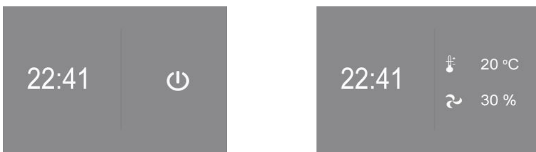
Figure 20. Control panel with touchscreen display in standby mode: the Unit is switched off, the Unit is in operation
