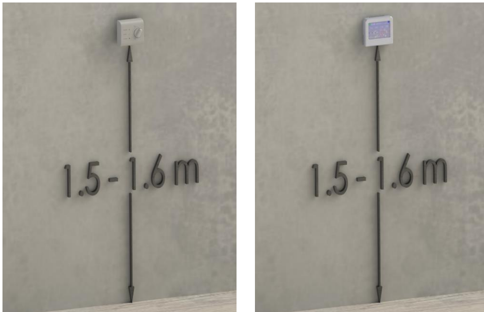
Figure 6. Installation of the control panel
