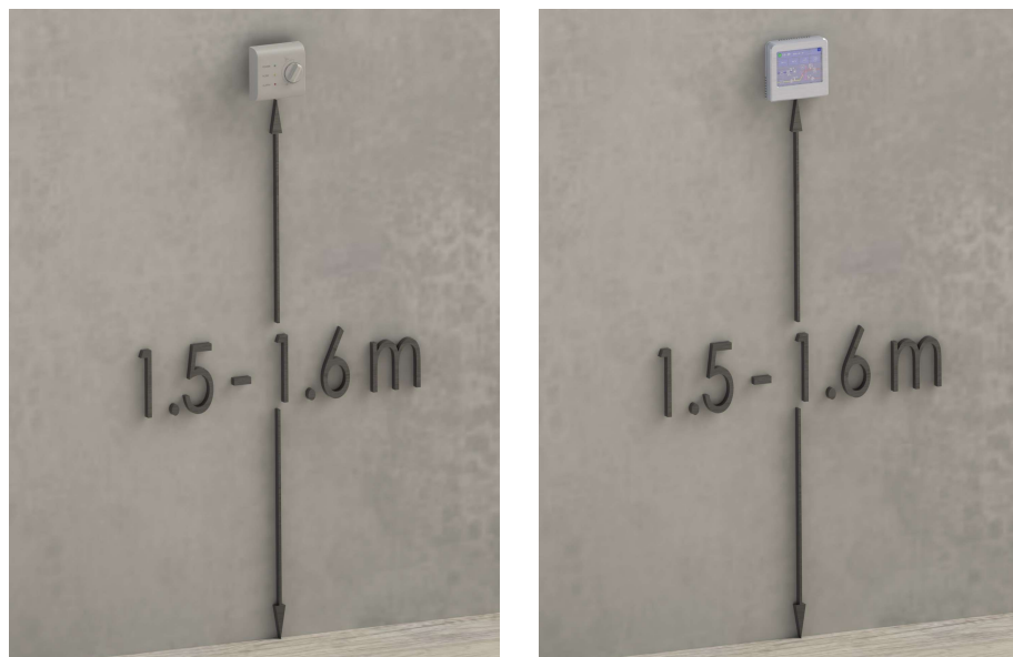
Figure 9. Installation of the control panel
