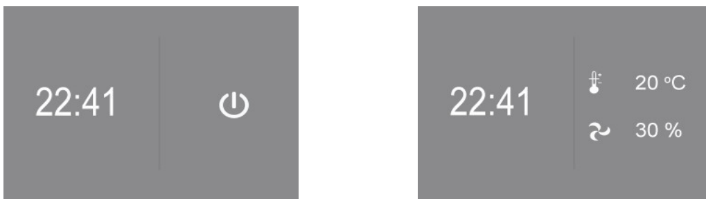
Figure 23. Control panel with touchscreen display in standby mode: the Unit is switched off, the Unit is in operation
