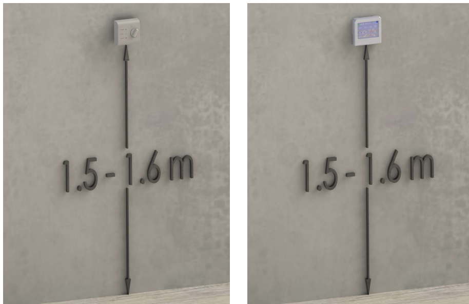
Figure 6. Installation of the control panel
