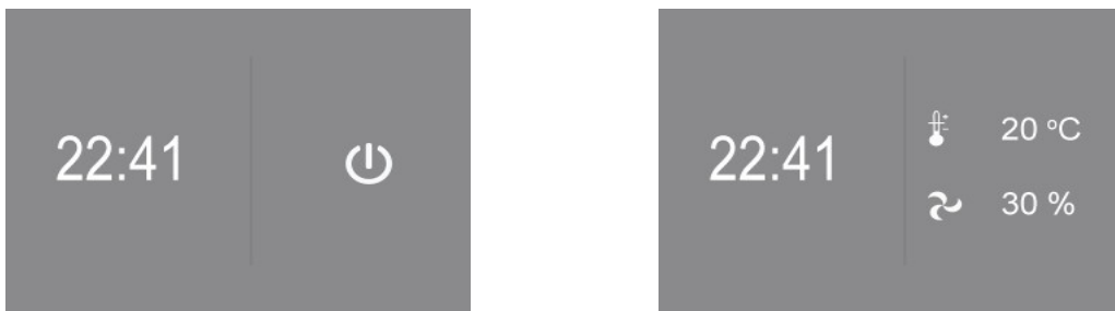
Figure 22. Control panel with touchscreen display in standby mode: the Unit is switched off, the Unit is in operation
