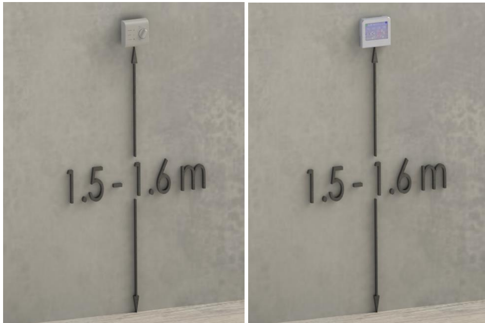
Figure 5. Installation of the control panel
