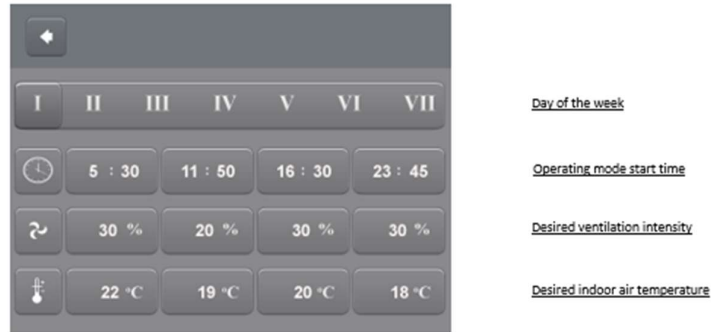
Figure 23. Weekly operating mode settings menu
