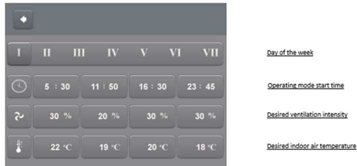
Figure 23. Weekly operating mode settings menu
