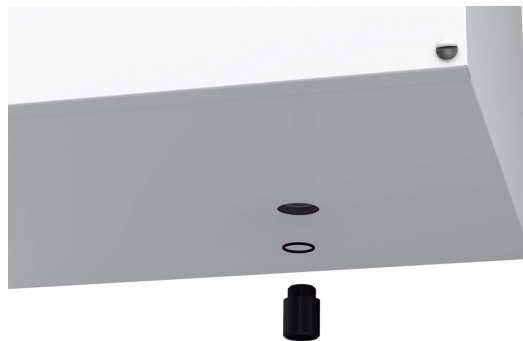
Figure 4. Installing the condensate drain
